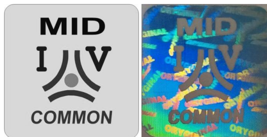
Figure 8.4 patten and view of primary verification marking
