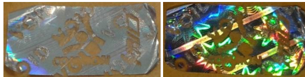
Figure 8.3 view of broken metrological mark
