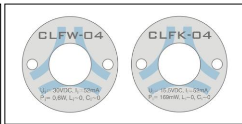
Fig. 15b Transmitters name plates
